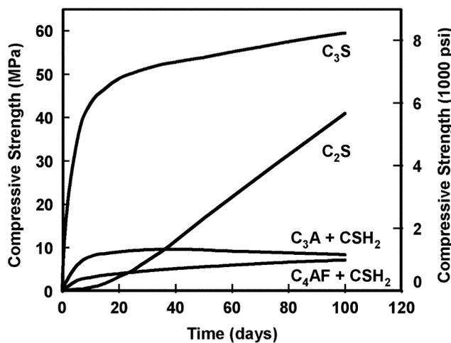
**Fig. 4.1—Contribution of cement compounds to strength development.<sup>18</sup>**
