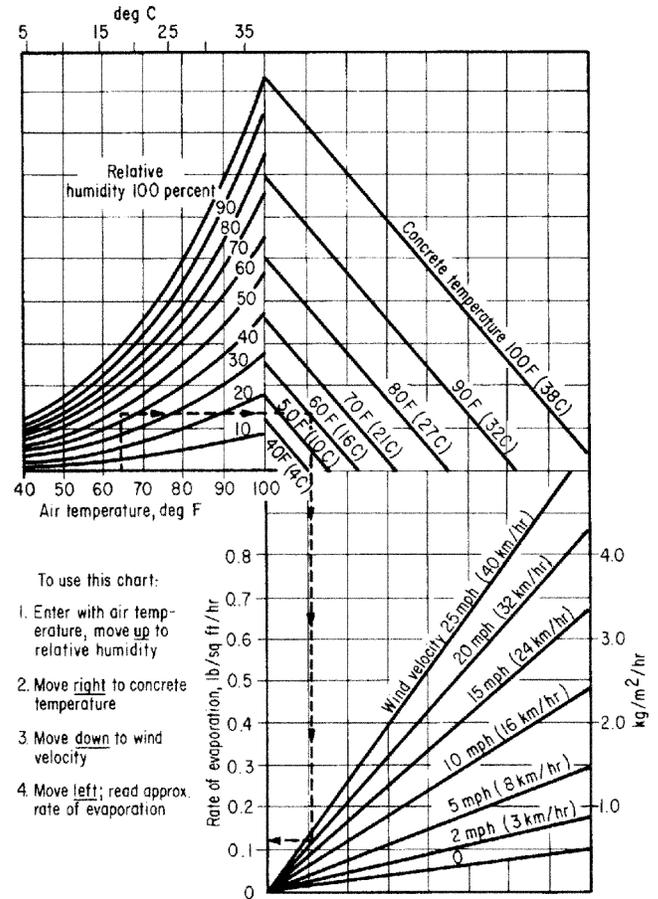
Fig. 5.2—Chart to calculate evaporation rate under prevailing environmental and concrete temperature conditions.<sup>3</sup>
