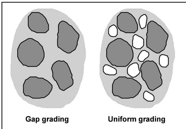
Fig. 4.3—Diagram showing how intermediate blend size aggregates fill spaces between larger, coarse aggregates.
