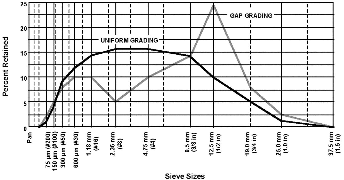
Fig. 4.2—Grading plot showing gap-graded mixture and mixture with adequate intermediate particles.
